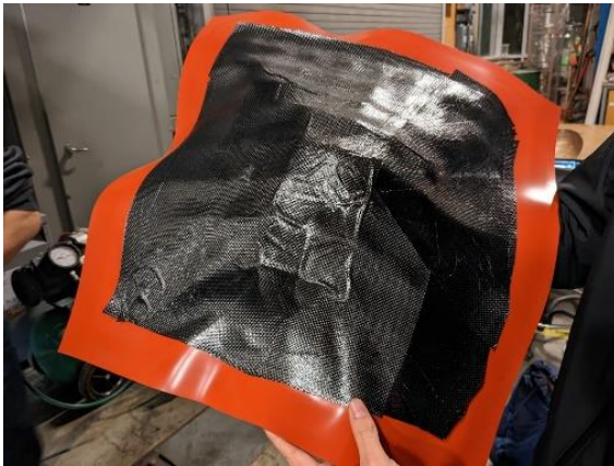
Figure 15, Finished part and laying up carbon fibre
