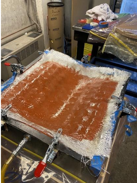
Figure 16, Layup and finished fibreglass product
