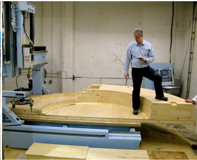
Figure 18. Tim Olson of Adanac Patterns, machining solid wood molds (From Adanac Patterns website)
